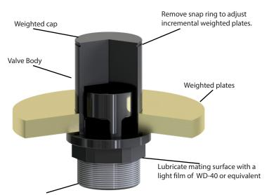
Use Teflon Tape on all threads (Hand-tighten in order to prevent deformation or galling of aluminum threads.)
